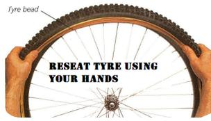
Starting at the valve hole, use your thumbs to push the tyre onto the rim.
