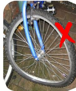
If the wheel catches the brake pads then it might be buckled and will need repairing by a mechanic.
