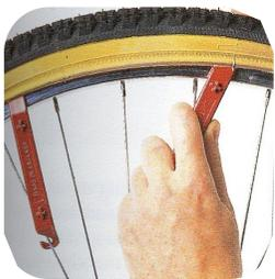
Insert the 2nd tyre lever under the tyre a few spokes from the 1st and slide it around lifting the tyre off the rim.
