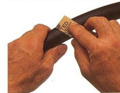
Spread solution onto tube so it is bigger than your patch.
