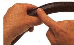
Wait until the solution is sticky, then apply the patch firmly to the tube.
