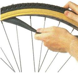
When one side of the tyre is loose, push the valve up into the tyre and pull the tube out of the tyre to remove it.
